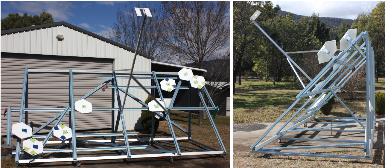
Figure 2. The model PWF collector. The four ersatz reflectors that have secondary mirrors at several vertices can be seen towards the lower left and upper right in the front view.
