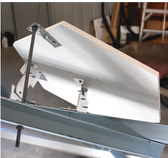
Figure 3. A threaded rod controls tilt of this reflector about its mounting axis, as a substitute for a linear actuator.
