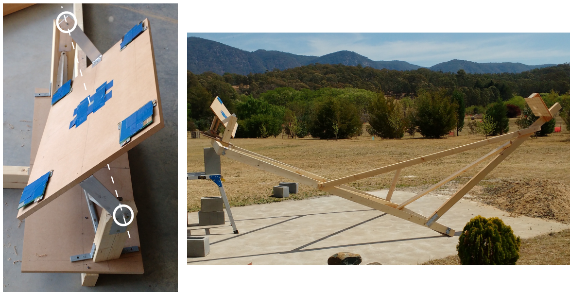
Figure 3. The 5/3-scale model (right), tilted towards the sun for higher apparent sun elevation, and the mirror unit (left). White circles indicate mirror mounting points.
