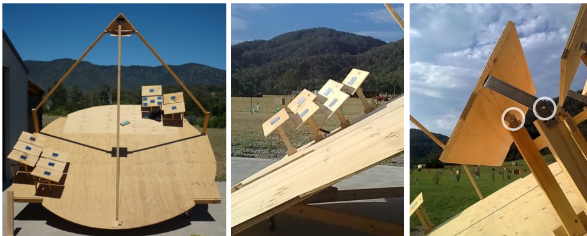
Figure 3. Physical model. (a) Sun elevation 60^\circ , mirror units aligned with paraboloidal surface. (b) Sun elevation 14^\circ , mirror units rotated to suit. (c) Typical axis of rotation for a mirror unit, defined by its mounting screws (circled).
