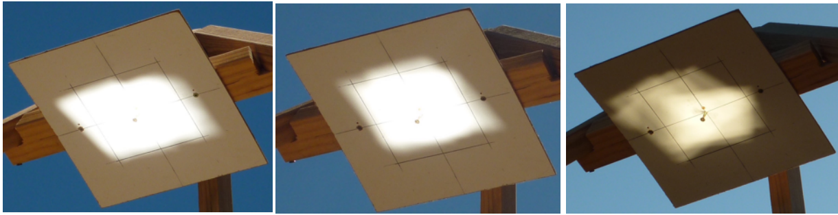
Figure 6. Images on the 300 x 300 mm target from 100 x 100 mm mirror tiles at the centres of 10 mirror units. Sun elevations (a) 78°, (b) 49°, (c) 9°.
