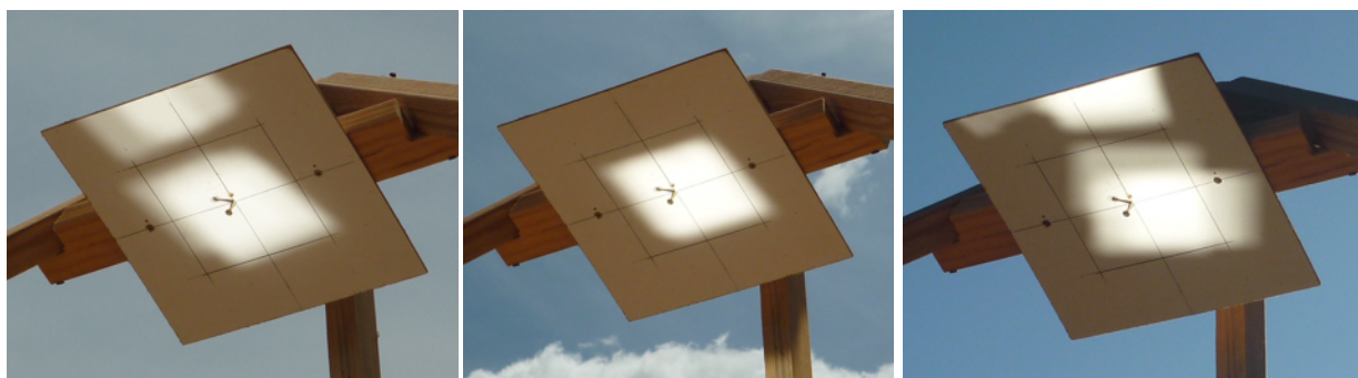
Figure 7. Images from the corner mirror tiles (plus centre) of Unit 3 at sun elevations (a) 78°, (b) 56°, (c) 16°. The additional patches of light come from other mirror units aimed slightly above the target.
